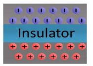
Static discharges can be harmful depending on what medium the charges travel through and to what surfaces the charges are transferring. Charges equalizing through an air gap can result in a visible shock as the traveling electrons collide with electrons in the air, which become excited and release energy in the form of light.
