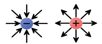
The electric fields of single charges. A negative charge has an inward electric field because it attracts positive charges . The positive charge has an outward electric field , pushing away like charges.
