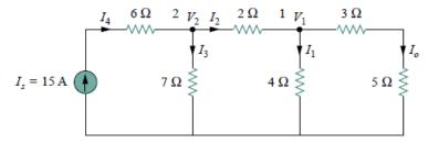
If  $I_o = 1$  A, then  $V_1 = (3+5)I_o = 8$  V and  $I_1 = \frac{v_1}{4} = \frac{8}{4} = 2$  A. Applying KCL at node 1 gives
