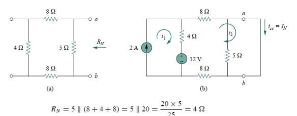
To find  $I_N$ , we short-circuit terminals a and b, as shown in Fig. (b). We ignore the  $5\Omega$  resistor because it has been short-circuited. Applying mesh analysis, we obtain
