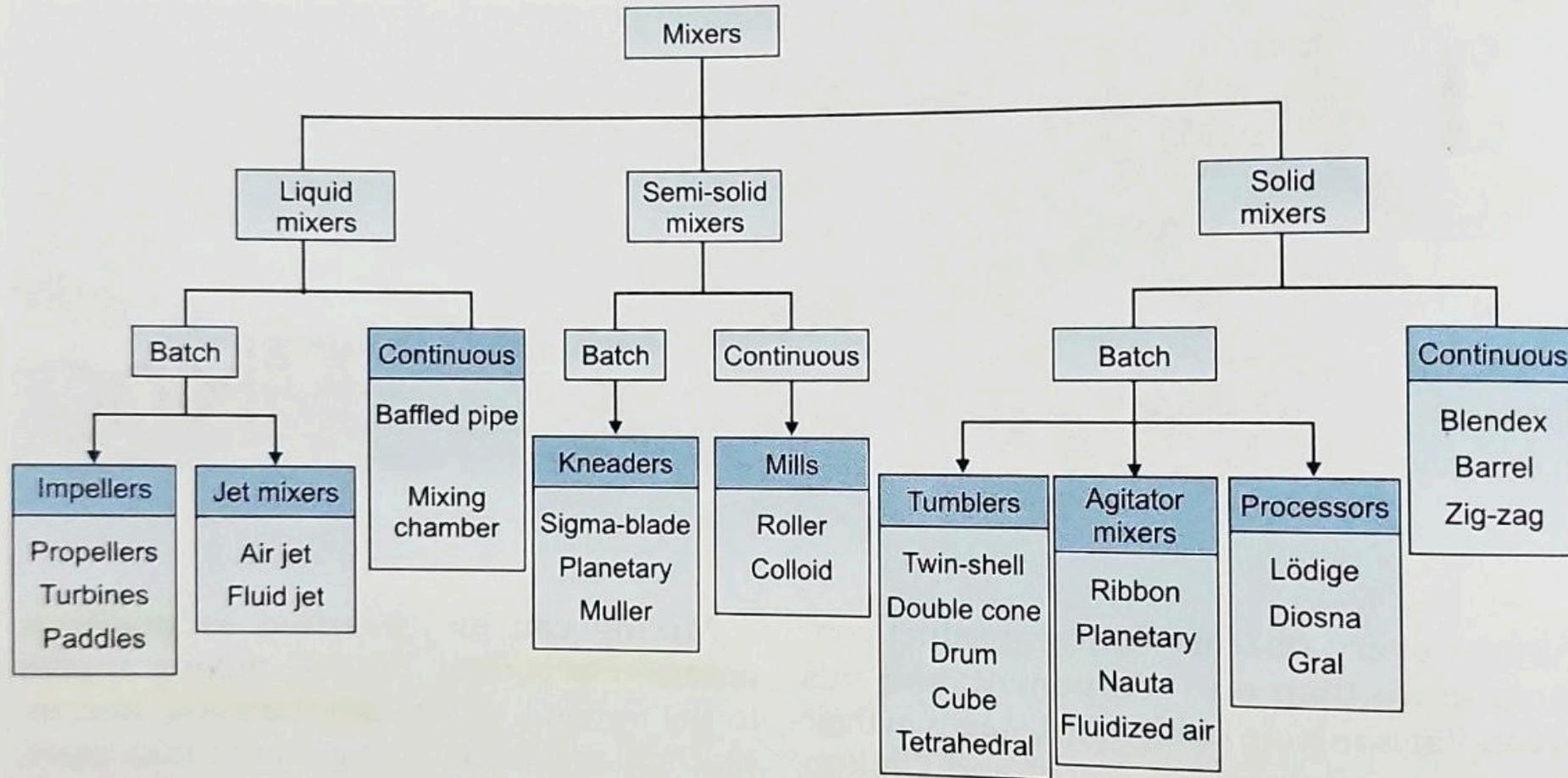
Fig. 1.1: Classification tree of mixing equipments
