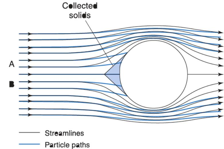
Fig. 25.1 • Filtration by impingement.
