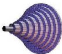
Figure 1. The area under f(x) , bounded by f(x) , x-axis, y-axis and the vertical line x=2 rotated about x-axis
