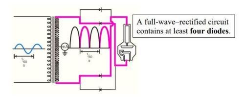
The half wave rectified x-ray tube emits x-rays only half of the time. The pulsed xray output of a full-wave—rectified machine occurs 120 times each second instead of 60 times per second as with half-wave rectification.
