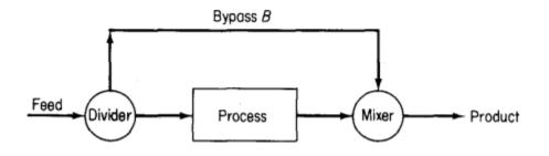
A bypass stream can be used to control the composition of a final exit stream from a unit by mixing the bypass stream and the unit exit stream in suitable proportions to obtain the desired final composition.
