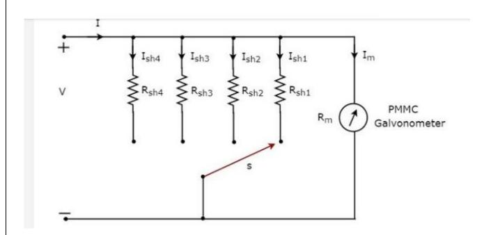
a) Direct Dc Ammeter Method (Ayton Shunt):
