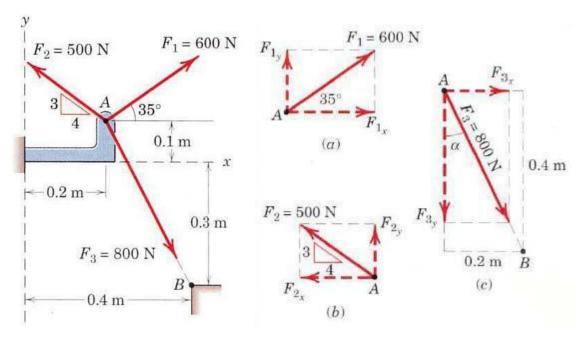
Solution: The scalar components of F1' from Fig. a, are
