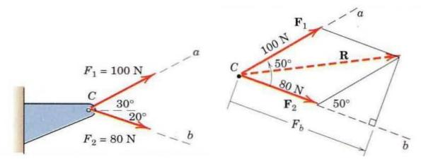
Solution. The parallelogram addition of F1 and F2 is shown in the figure. Using the law of cosines gives us R2 = (80)2 + (100)2 - 2(80)(100) cos 130
