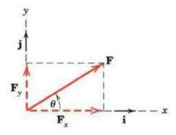
The scalar components can be positive or negative, depending on the quadrant into which F points.
