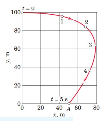
The velocity and acceleration components and their resultants are shown on the separate diagrams for point A, where y=0. Thus, for this condition we may write
