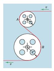
5/20 Point A of the circular disk is at the angular position θ = 0 at time t = 0. The disk has angular velocity ω<sub>0</sub> = 0.1 rad/s at t = 0 and subsequently experiences a constant angular acceleration α = 2 rad/s². Determine the velocity and acceleration of point A in terms of fixed i and j unit vectors at time t = 1 s.
