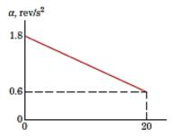
**5/28** The design characteristics of a gear-reduction unit are under review. Gear B is rotating clockwise with a speed of 300 rev/min when a torque is applied to gear A at time t=2 s to give gear A a counterclockwise acceleration  $\alpha$  which varies with time for a duration of 4 seconds as shown. Determine the speed  $N_B$  of gear B when t=6 s.
