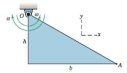
5/3 The body is formed of slender rod and rotates about a fixed axis through point O with the indicated angular properties. If ω = 4 rad/s and α = 7 rad/s², determine the instantaneous velocity and acceleration of point A.
