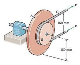
5/18 Magnetic tape is being fed over and around the light pulleys mounted in a computer. If the speed v of the tape is constant and if the magnitude of the acceleration of point A on the tape is 4/3 times that of point B, calculate the radius r of the smaller pulley.
