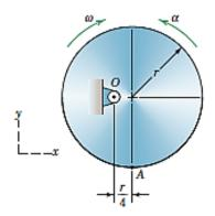
5/2 The triangular plate rotates about a fixed axis through point O with the angular properties indicated. Determine the instantaneous velocity and acceleration of point A. Take all given variables to be positive.
