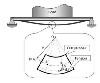
Consider a fiber at a distance y from the neutral axis, because of the beam's curvature, as the effect of bending moment, the fiber is stretched by an amount of cd. Since the curvature of the beam is very small, bcd and oba are considered as similar triangles. The strain on this fiber is:
