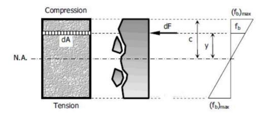
Considering a differential area dA at a distance y from N.A., the force acting over the area:
