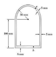
A 5.6 kN m torque is applied to a hollow shaft having the cross section shown. Neglecting the effect of stress concentrations, determine the shearing stress at points a and b.
