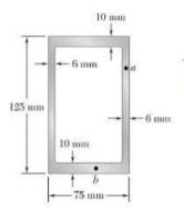
A torque  $T = 5 \text{ kN} \cdot \text{m}$  is applied to a hollow shaft having the cross section shown. Neglecting the effect of stress concentrations, determine the shearing stress at points a and b.
