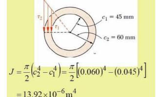
$$\frac{\tau_{\min}}{\tau_{\max}} = \frac{c_1}{c_2} \qquad \frac{\tau_{\min}}{86.2 \,\text{MPa}} = \frac{45 \,\text{mm}}{60 \,\text{mm}}$$
