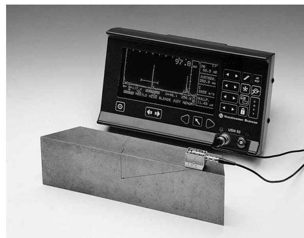
Fig. 55 USN 50: A hole being scanned with the probe MWB 60-4E
