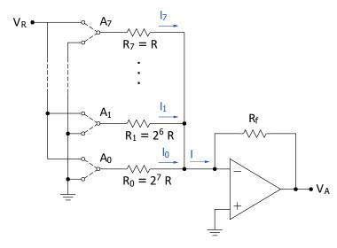
\* If  $R_f = R$ , what is the resolution (i.e.,  $\Delta V_A$  corresponding to the input LSB changing from 0 to 1 with other input bits constant)?
