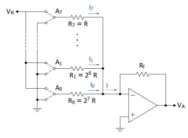
\* Find the output voltage corresponding to the input 1010 1101.
