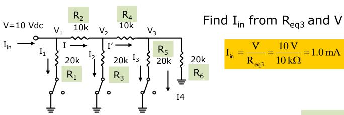
$$I_{in} = \frac{V}{R_{gas}} = \frac{10 \text{ V}}{10 \text{ k}\Omega} = 1.0 \text{ mA}$$
