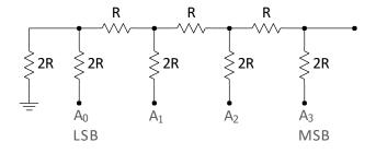
Node  $A_k$  is connected to  $V_R$  if input bit  $S_k$  is 1; else, it is connected to ground.
