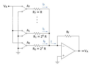
\* If the resistors are specified to have a tolerance of 1%, what is the range of  $|V_A|$  corresponding to input 1111 1111?
