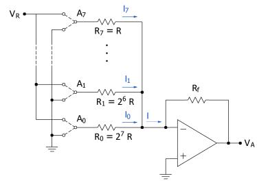
\* Consider an 8-bit DAC with  $V_R = 5$  V. What is the smallest value of R which will limit the current drawn from the supply  $(V_R)$  to 10 mA?
