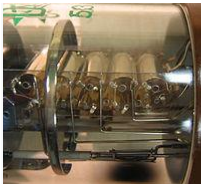
Dynodes inside a photomultiplier tube
