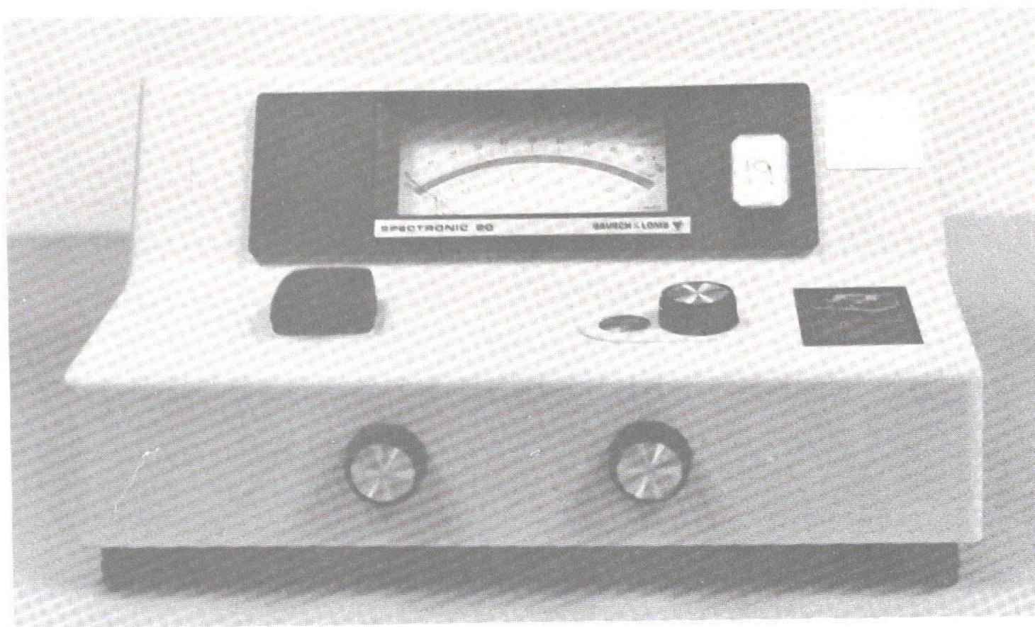
Figure 7-5. An example of a spectrophotometer (Photo by John Estridge)
