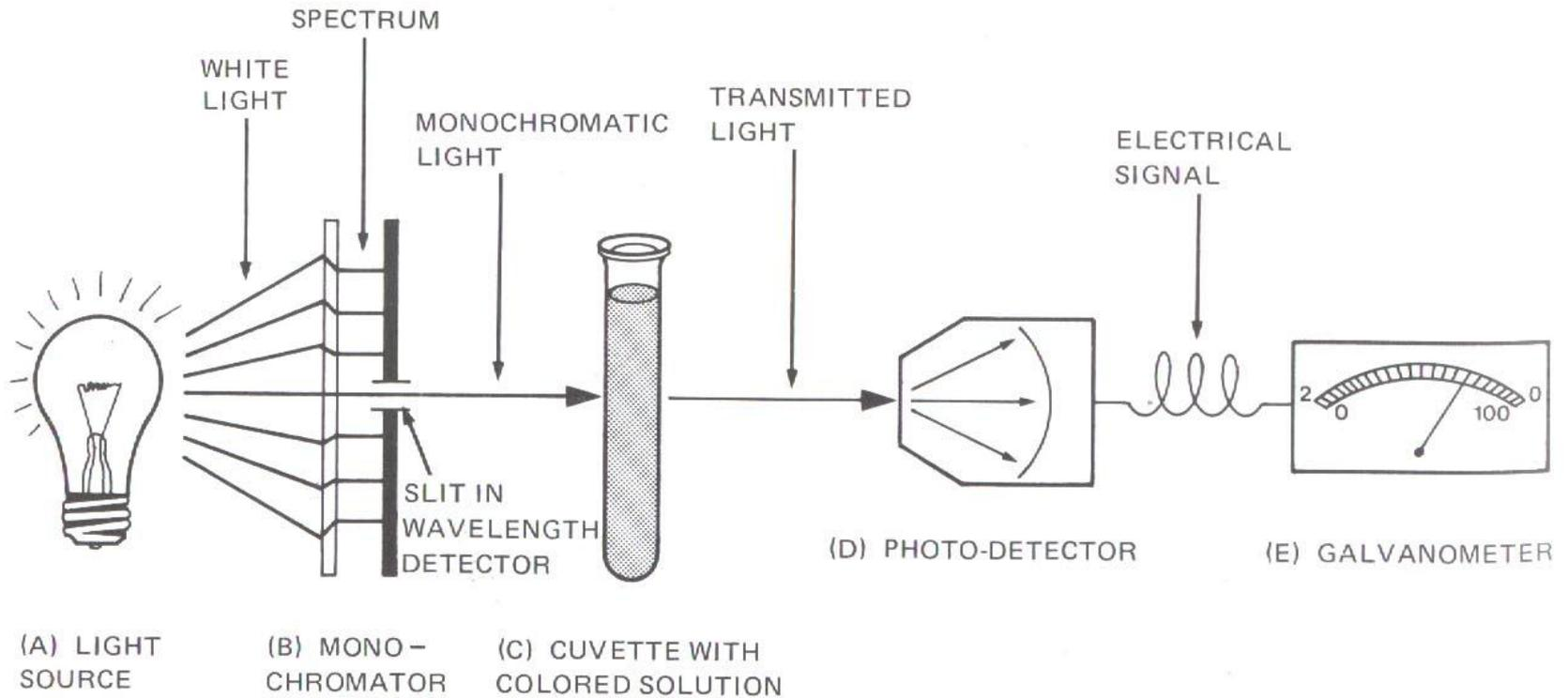
Figure 7-6. Diagram of internal parts of a spectrophotometer
