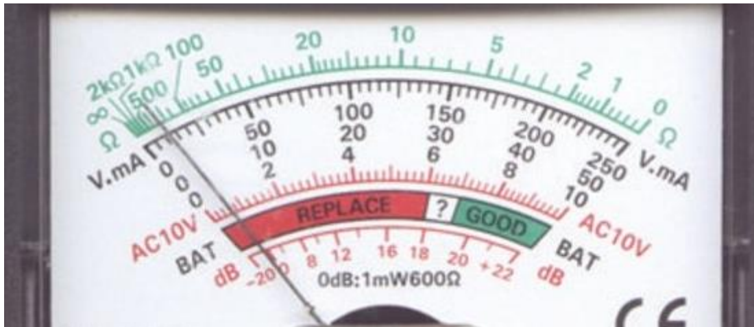
Figure 7.2 The arrangement of the scale of series type ohmmeter
