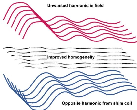
Figure 5: Theory underlying active shimming. Unwanted harmonics in the inhomogeneous field are canceled/neutralized by a shim component of equal and opposite polarity.
