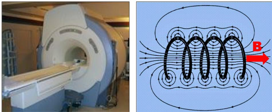
Figure 6. **Left:** superconducting scanner, **right:** Magnetic field created by solenoid
