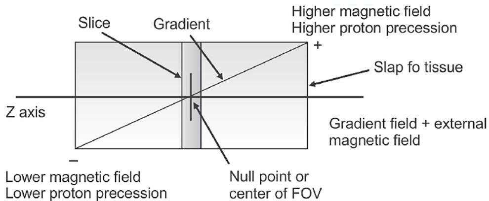
**Figure 4:** Gradient magnetic field makes the proton slower at the toe side and faster at the head side and moderate precession at the middle (null point).
