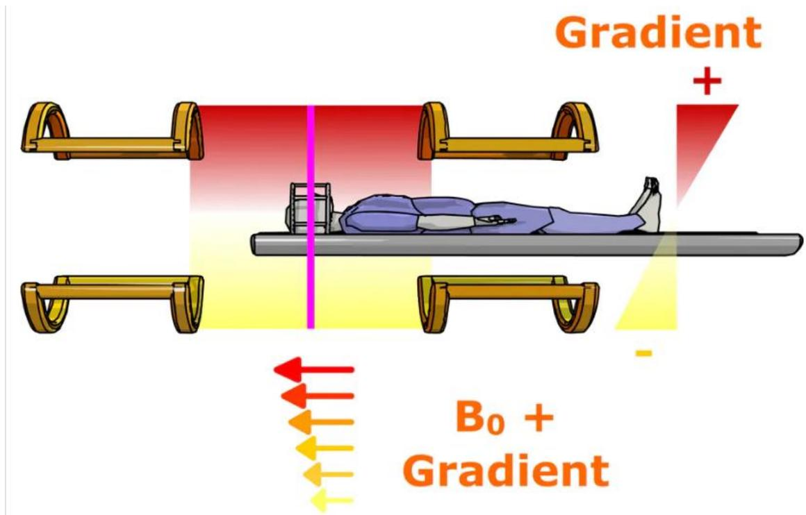
**Figure 5:** Y-axis gradient coil, for phase encoding gradient.
