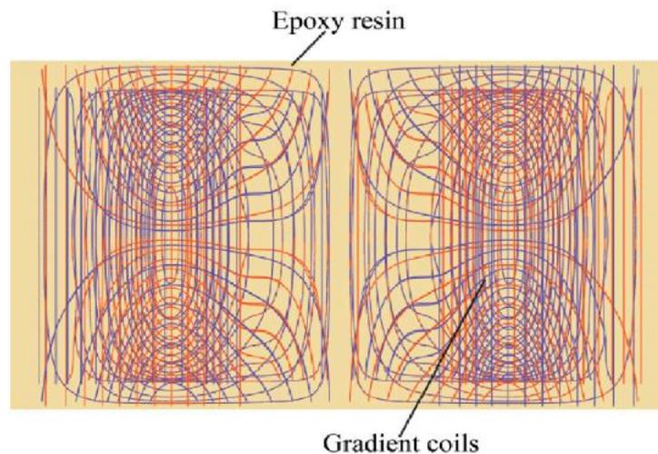
Figure 2: Illustration of the three-axis gradient coils fixed in the epoxy resin.
