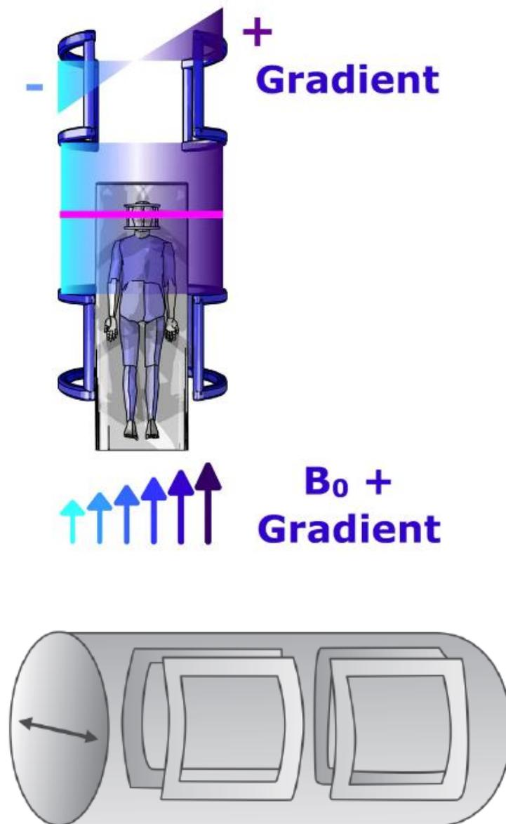
**Figure 7:** X-axis gradient coil, for frequency encoding
