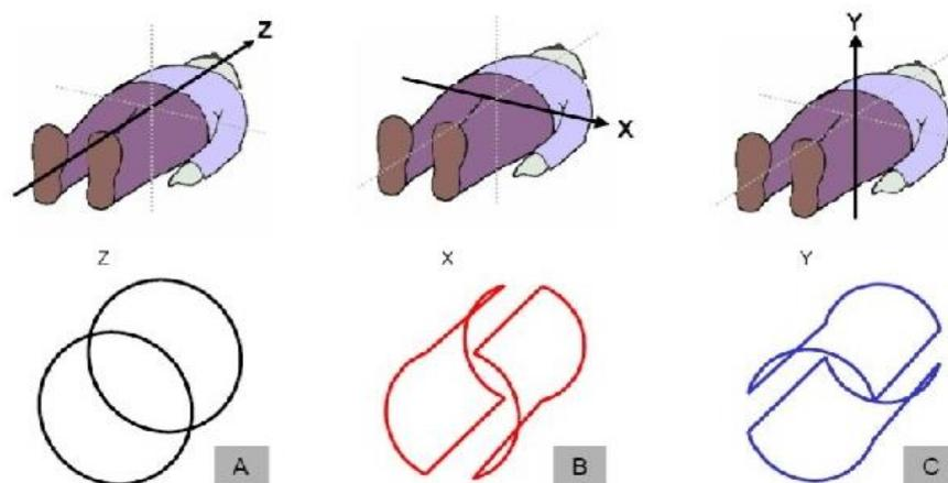
**Figure 1B:** shows three sets of wires. Each set creates magnetic field in a specific direction: Z, X and Y.
