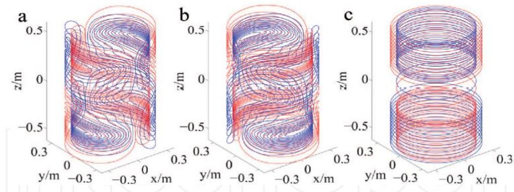
**Figure 1A:** Actively shielded gradient coils used in an MRI scanner: (a) x gradient coil, (b) y gradient coil, and (c) z gradient coil. The red and blue colors indicate the direction in which the current flows.
