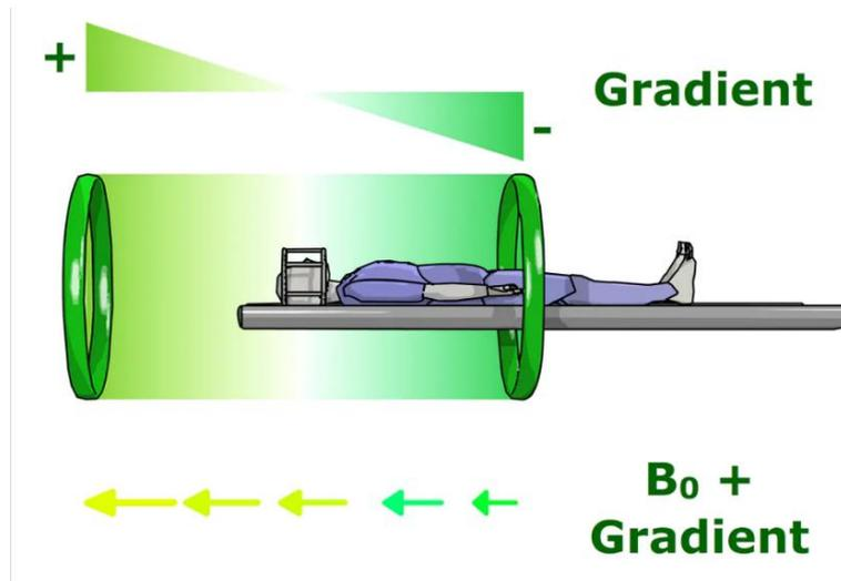
**Figure 3:** Z axis gradient coil, for slice selection
