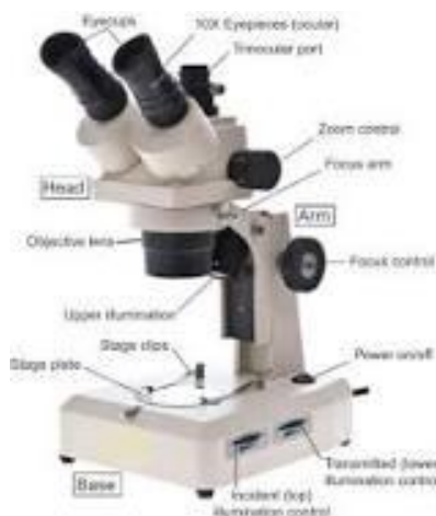
Figure 1: light microscope parts
