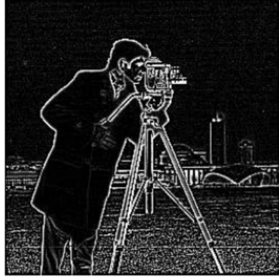
(b) Laplacian of Gaussian ("log") filtering
