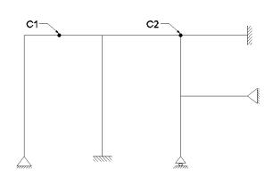
r > C+3, the frame is stable & indeterminate  $5^{th}$  degree.
