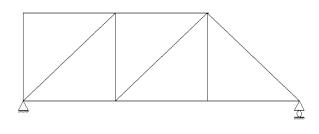
The truss is stable &determinate
