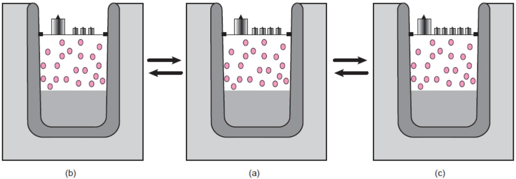
reversible process: evaporation and condensation of water at 1 atm in a closed system.
