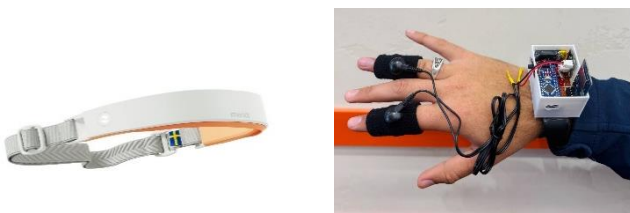
fNIRS headband and EDA device.
