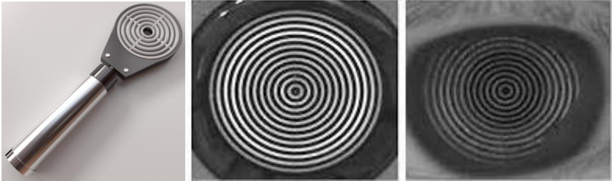
Figure 6. Placido disc ring patterns – normal vs astigmatic cornea
