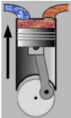
d- Piston moves up compressed vapour
