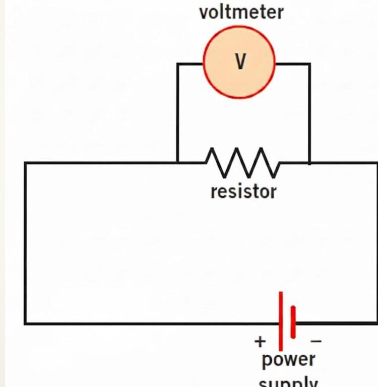
Measuring voltage with the voltmeter ( $V$ ) in parallel across two points
