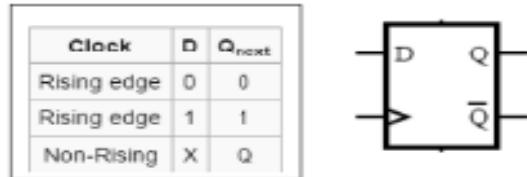
The data bus lines connected the D-input and the Q-output is connected to the destination. The controller generates a control signal applied at the CLK of the flip flop to latch data from D to Q.
