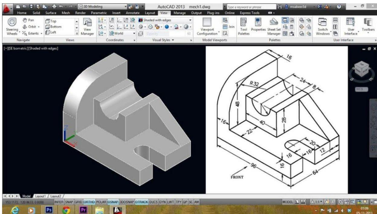
This is a screenshot of a 3D CAD environment. It shows a mechanical part being modeled in 3D. On the sides, you see toolbars with functions for drawing, modifying, measuring, and analyzing the model. This interface is typical of programs like AutoCAD, Solid Works.
