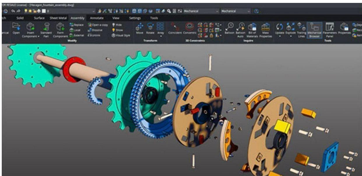
This image shows an exploded view of a mechanical assembly in a CAD program (BricsCAD Mechanical). Each component is pulled apart slightly to show how they fit together. This view is useful for understanding the internal structure of complex products .
