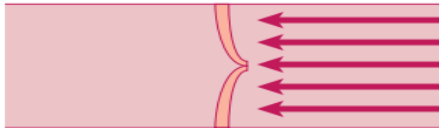
Valve closed; does not open in opposite direction
