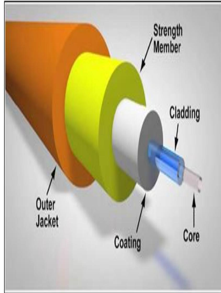
When the light enters one end of the optical fiber , it travels from a dense medium towards rare medium with a finite angle. The light ray hits the core-cladding interface with an angle greater than the critcl angle and thus gets refelected at the interface due to total internal reflection. It suffers multiple total internal refelection the whole length of the fiber and finally emerges out of the other end of the fiber.
