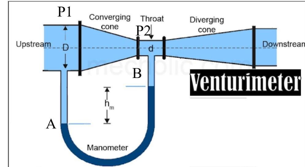
Determine the pressure head between inlet and throat
