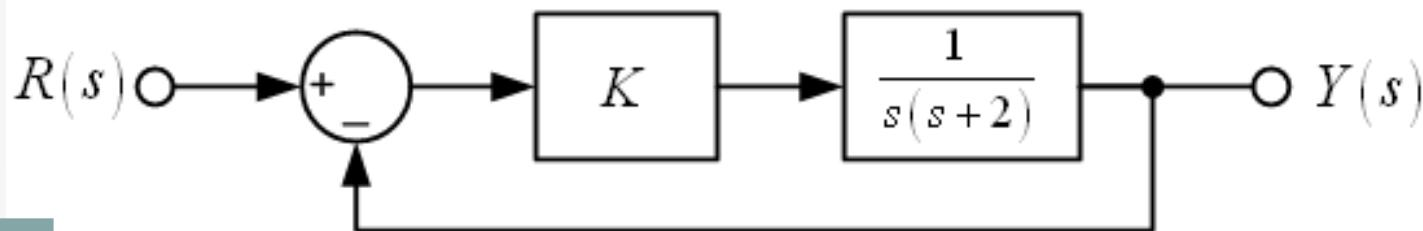
$$\frac{Y(s)}{R(s)} = \frac{\frac{K}{s(s+2)}}{1 + \frac{K}{s(s+2)}} = \frac{K}{s^2 + 2s + K} \Rightarrow 2\zeta\omega_n = 2 \\ \Rightarrow \omega_n^2 = K$$
