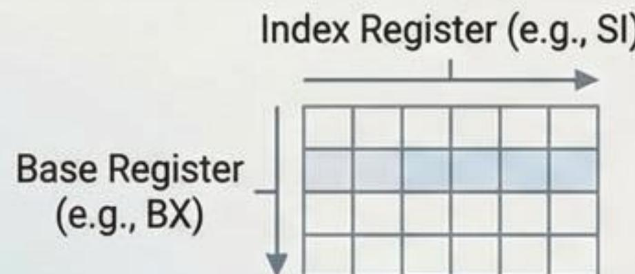
Efficiently facilitates 2-D array traversal. The **Base Register** typically points to the row, while the **Index Register** points to the column within that row.
