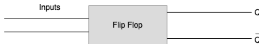
Figure 1 The S and R in SR flip-flop mean 'SET' and 'RESET' respectively.
