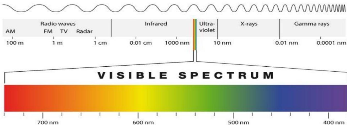
These spectra are generally characterized as they are produced when a molecular or atomic group transitions from a quantum state with a certain energy level to a quantum state with a lower energy level.
