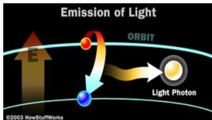
Although there are many types of lasers, all have certain essential features. In a laser, the lasing medium is “pumped” to get the atoms into an excited state. Typically, very intense flashes of light or electrical discharges pump the lasing medium and create a large collection of excited-state atoms (atoms with higher-energy electrons). It is necessary to have a large collection of atoms in the excited state for the laser to work efficiently.
