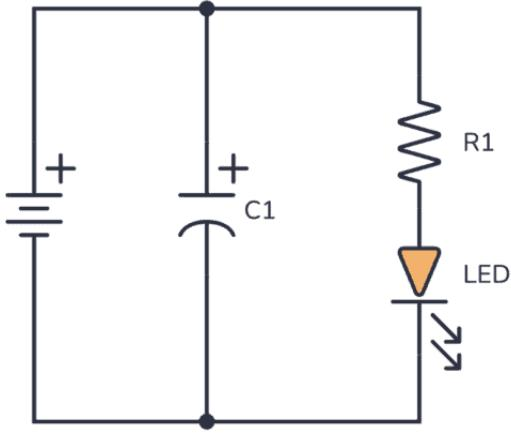
Capacitors store energy using electric potential difference.
