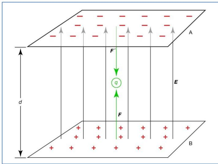
The diagram shows how electric potential decreases in the direction of the electric field.
