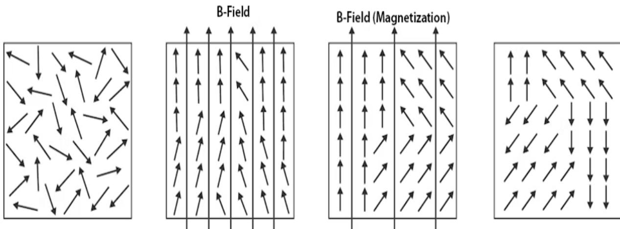
In the image, the magnetic moments of the electron spins are represented by small arrows. Long arrows that extend beyond the boundary of the images indicate a resulting magnetic flux density in the entire material, i.e. a magnetic field. In this case, we speak of a macroscopic flux density. Without an external magnetic field, the spins of a paramagnetic material are randomly orientated (left image). The overall magnetisation is
