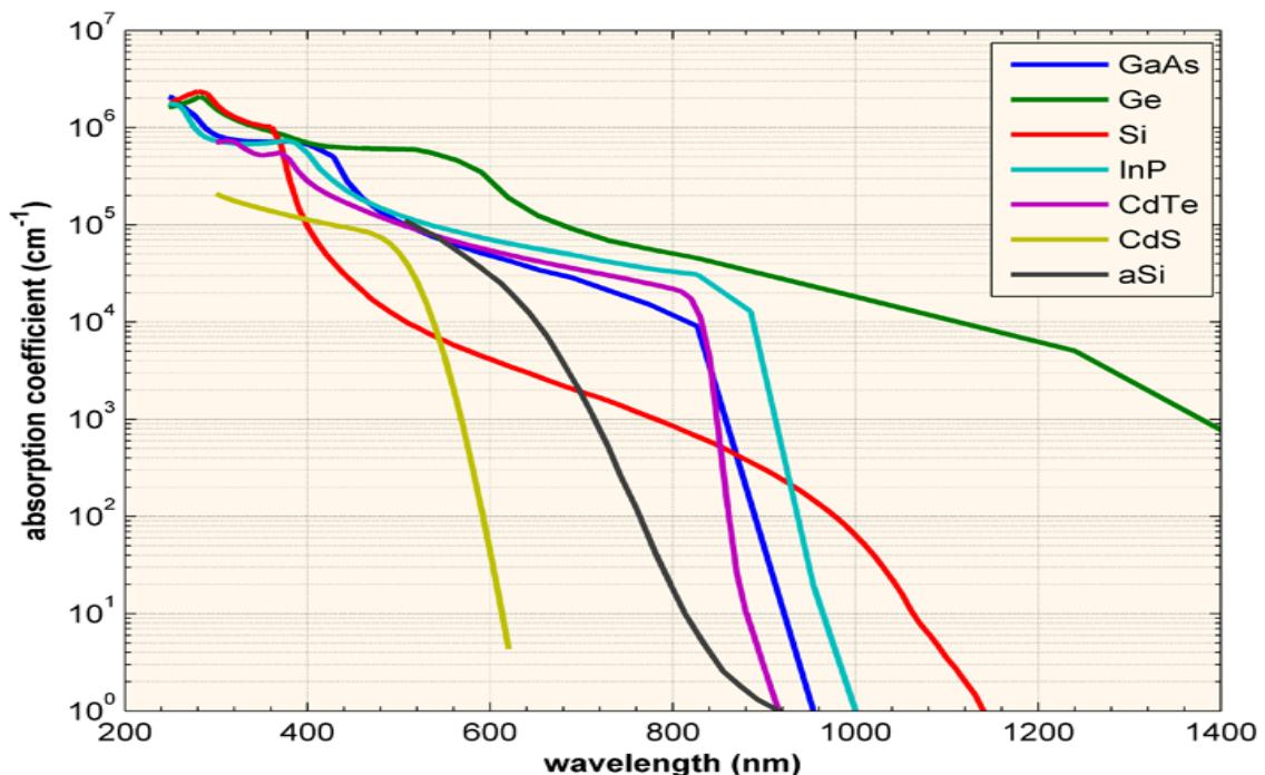
*The absorption coefficient,  $\alpha$ , in a variety of semiconductor materials at 300K as a function of the vacuum wavelength of light.*
