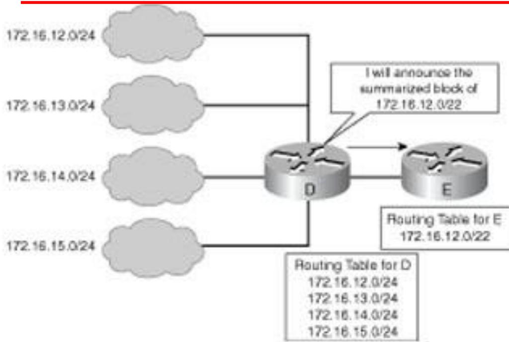
Router D can either send four routing update entries or summarize the four addresses into a single network number. If router D summarizes the information into a single network number entry, the following things happen:
