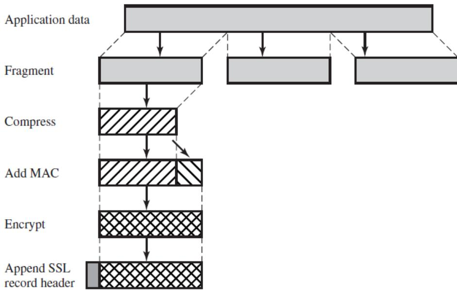
Figure /SSL Record Protocol Operation
