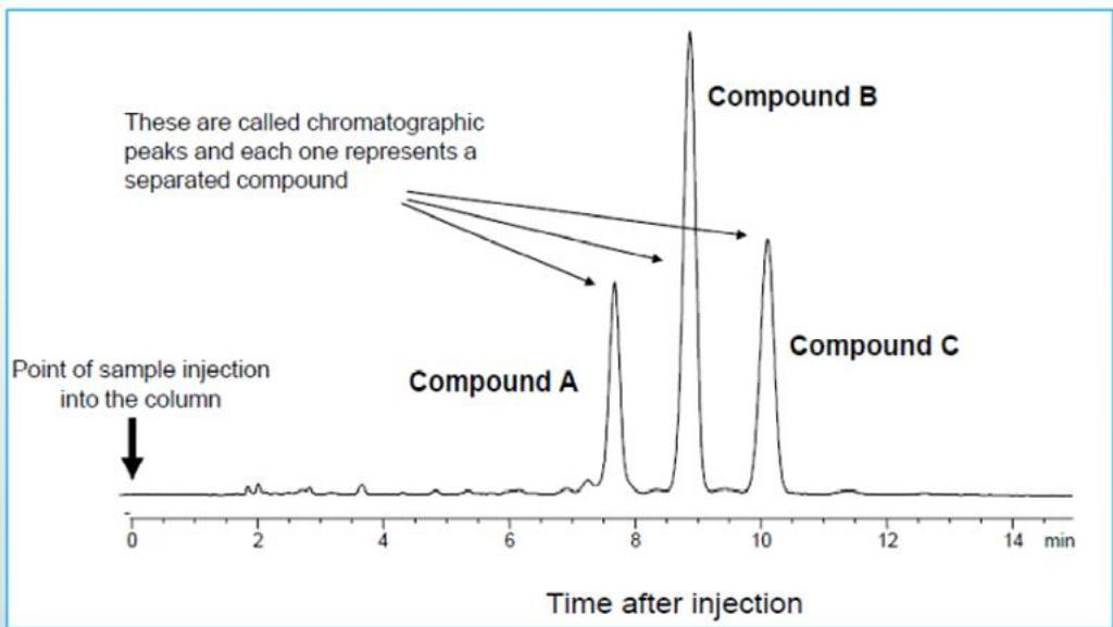
This is the chromatogram resulting from the injection of a small volume of liquid extracted from a vitamin E capsule that was dissolved in an organic solvent. Modern HPLC separations usually require 10-to 30-minutes each.
