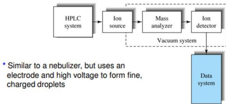
F) Computer: Frequently called the data system, the computer not only controls all the modules of the HPLC instrument but it takes the signal from the detector and uses it to determine the time of elution (retention time) of the sample components (qualitative analysis) and the amount of sample (quantitative analysis).
