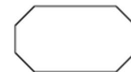
Specify second chamfer distance for rectangles<0.000>: in y direction
