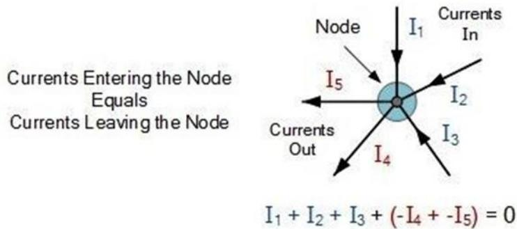
Here, the three currents entering the node,  $I_1$ ,  $I_2$ ,  $I_3$  are all positive in value and the two currents leaving the node,  $I_4$  and  $I_5$  are negative in value. Then this means we can also rewrite the equation as:
