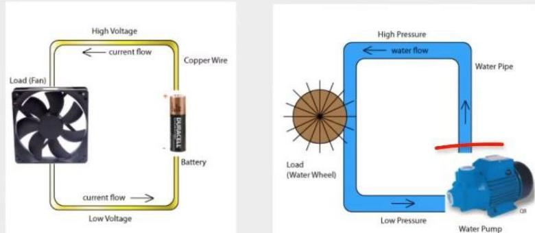
Then all basic electrical or electronic circuits consist of three separate but very much related electrical quantities called: **Voltage**, ( **V** ), **Current**, ( **i** ) and **Resistance**, (  **$\Omega$**  )
