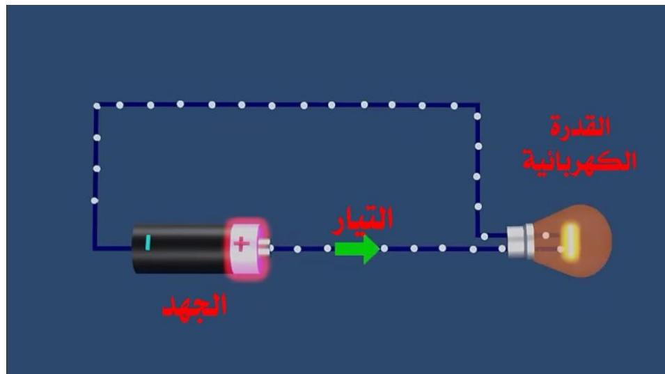
Current is measured in **Amps** and an amp or ampere is defined as the number of electrons or charge (Q in Coulombs) passing a certain point in the circuit in one second, (t in Seconds).
