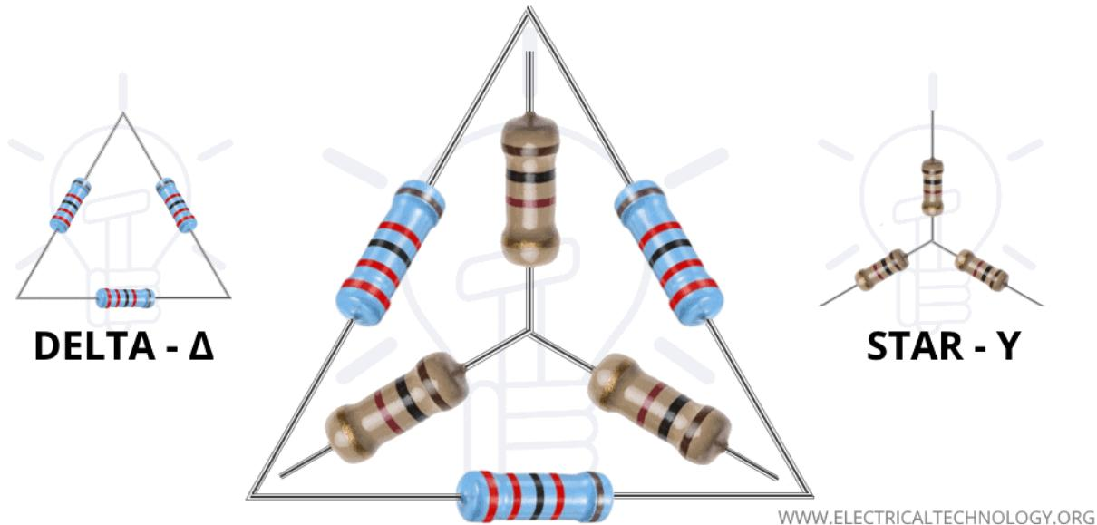
To solve complex electrical networks or simplify it, we use the star-delta conversion technique. It replaces any star connected network with its equivalent delta connected network & vice versa.
