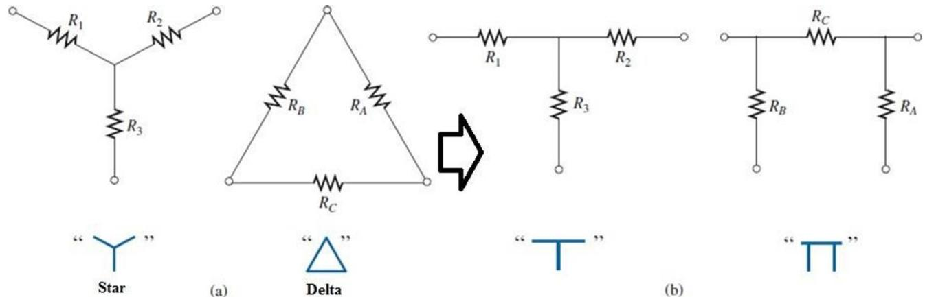
The given figure shows a delta network having A, B, C terminals with the impedances  $R_1$ ,  $R_2$ ,  $R_3$ . The equivalent star connected network with  $R_A$ ,  $R_B$  &  $R_C$  where they are connected to their corresponding terminals as shown in the figure.
