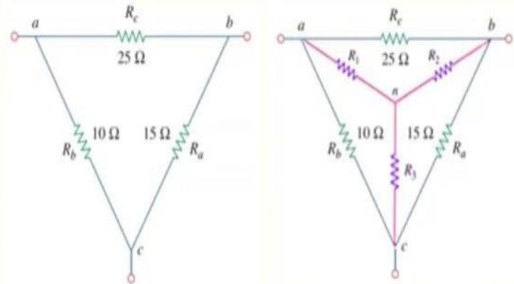
$$R_1 = \frac{R_b R_c}{R_a + R_b + R_c} = \frac{10 \times 25}{15 + 10 + 25} = \frac{250}{50} = 5 \Omega$$
